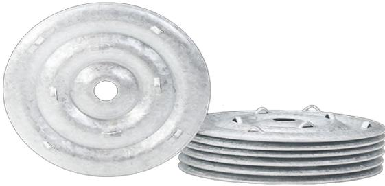
2-3/8" Barbed Metal Seam Plates are used to fix reinforced single-ply and modified bituminous membranes to the substrate. Used with #14 #15, purlin, fluted concrete nail or 1/4" concrete spike fasteners in roofing system applications.
