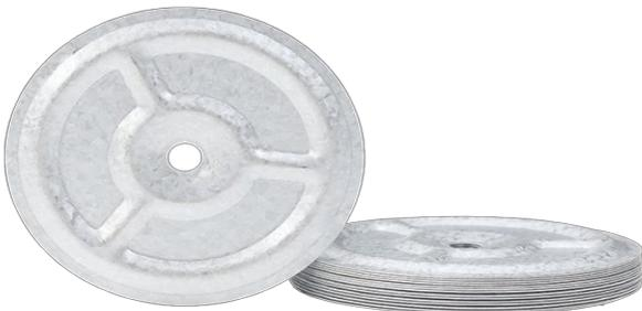
3" Metal Seam Plate is used within fully bonded seams to attach reinforced and non-reinforced single-ply membranes to the substrate. Used with #14 #15, purlin, fluted concrete nail or 1/4" concrete spike fasteners in roofing system applications.
