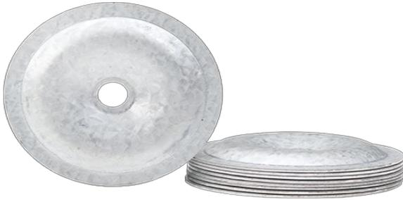
2" Metal Seam Plate is used within fully bonded seams to attach reinforced and non-reinforced single-ply membranes to the substrate. Used with #14 #15, purlin, fluted concrete nail or 1/4" concrete spike fasteners in roofing system applications.
