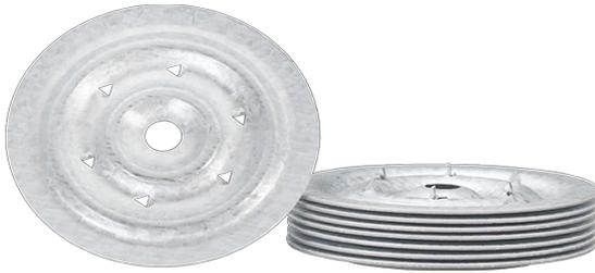
2-3/8" Barbed Metal Seam Plates are used to fix reinforced single-ply and modified bituminous membranes to the substrate. Used with #14 #15, purlin, fluted concrete nail or 1/4" concrete spike fasteners in roofing system applications.
